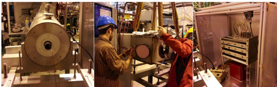
Figure 6.24: Photograph of the installation of different beam line elements: the decelerator (left), CEC chamber (center), and HV cage (right) .
