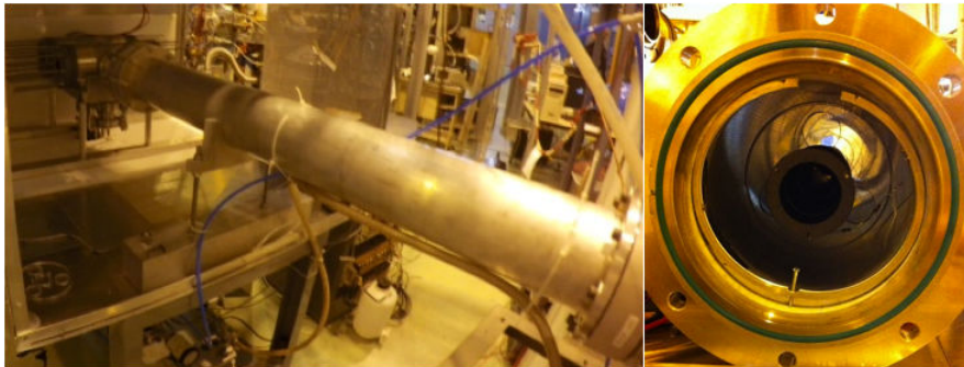
Figure 6.23: Photograph of the optical pumping region installed at the COLLAPS beam line. The pumping tube connected to the light collection region (left), and a view inside the pumping tube (right).
