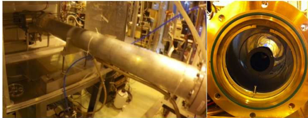
Figure 17: Photograph of the optical pumping region installed at the COLLAPS beam line. The pumping tube connected to the light collection region (left), and a view inside the pumping tube (right).
